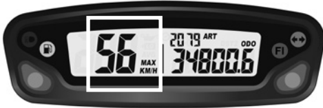
Fig 2 MAX speed function
