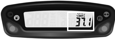
Fig 6 Adjustable trip distance function
