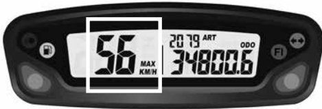
Fig 2 MAX speed function
