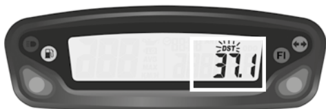
Fig 6 Adjustable trip distance function
